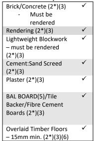
\*Substrates and considerations for priming - outside the use of BAL PRIMER 1C, prior to applying BAL WATERPROOF 1C - do not apply.
