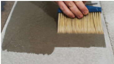
CONCRETE checking absorption
