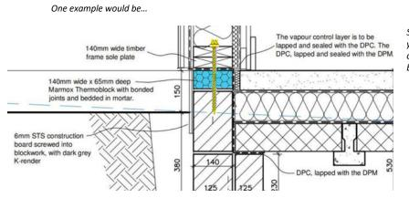
Screw, bolt or resin fixing (shown in yellow) penetrating through the centre of the Thermoblock (shown in blue) into the blockwork below
