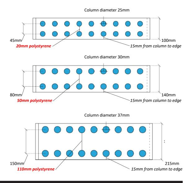
When fixed below timber frames, metal frames or door frames, screws and bolts must avoid the block edges where the concrete columns are located
