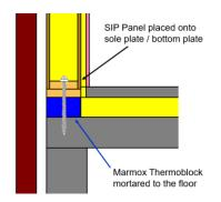
Screw, bolt or resin fixing penetrating through the centre of the Thermoblock (shown in blue) into the blockwork below.
