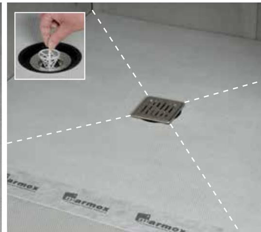
**12** There is no need to prime the unit, simply tile with cement-based tile adhesive. If tiles > 10cm, they should be cut along the lines shown.
