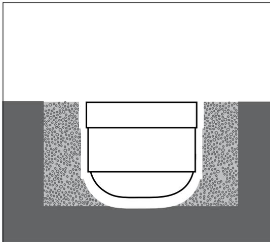
**2** The drain does not need supporting but the Showerlay does, so if the diameter void is wider than 130mm, in-fill with concrete.
