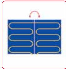
Turn the mesh through 180° parallel to the first run
