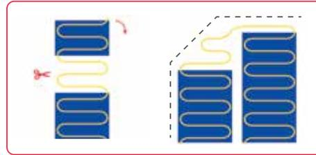
Remove the cable from the mesh and tape\* in place for awkward areas such as angled walls
