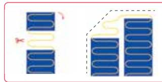
Remove the cable from the mesh and tape\* in place for awkward areas such as angled walls. \*Use small pieces of tape (max 10mm) and ensure there are no air voids around the cable.
