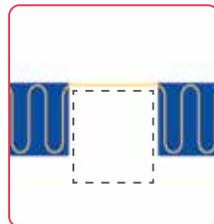
Remove the mesh to avoid permanent fixtures
