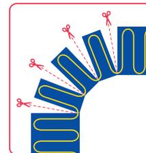
Cut mesh into sections to make a curved turn
