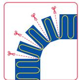
Cut mesh into sections to make a curved turn
