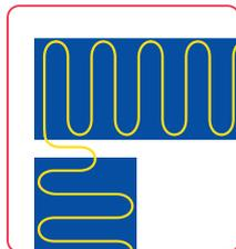
Release cable from the mesh for an alternative 90° turn
