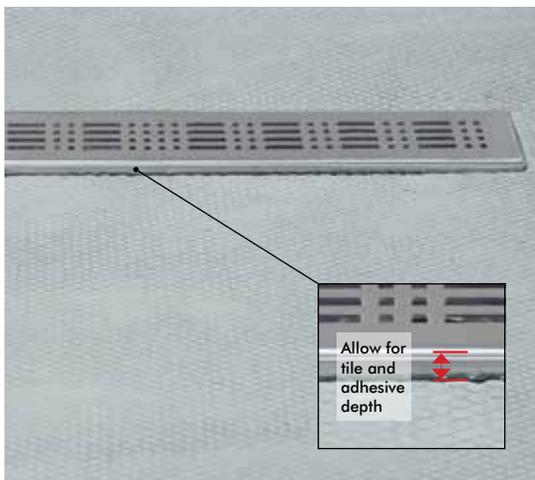
**6** The grate needs to be flush with the tiled surface (tile + adhesive). Raise the whole drainage channel using the 2mm and 4mm self-adhesive spacers.
