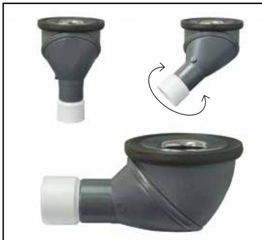
**3** Twist the drain to adjust the angle of the exit pipe if necessary to achieve the most suitable gradient.
